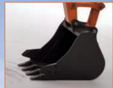
**Clamp Ready**Durable clamp mounts are integrated into the arm. There's no welding required to add a clamp.
